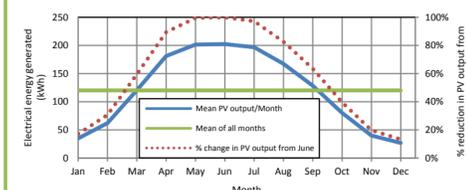
Figure 3. Average monthly electrical energy generation pattern of 18 PV system with a mean system size=2.33kWp, indicating percentage variation relative to the best performing month of June
