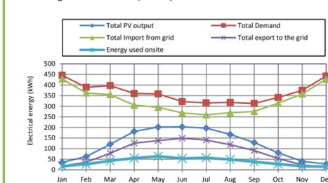
Figure 7. Comparison of the average monthly electrical energy demand, PV generation, electricity import and export of 18 households with a mean installed PV system size of 2.33kWp.
