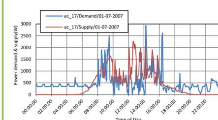
Figure 6. Comparison of the 5 minutely generation and demand patterns of a single household for: a) the days of 01-07-2007
