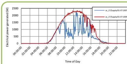
Figure 2. Illustration of intermittency in the electrical power generation pattern of a 3kWp PV system recorded on 1<sup>st</sup> July 2007 and 1<sup>st</sup> July 2009
